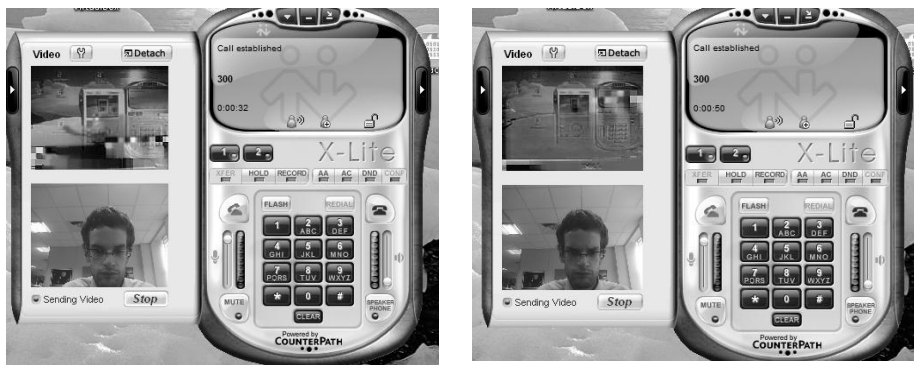
Figure 5 – Video call with 10% and 15% packet loss
